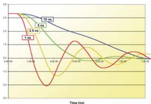
Figure 2 – The effect of driver edge rates on a 5 inch trace. The 10 ns and 5 ns edges look fine, with reflections and ringing effects appearing on the receiver waveforms for the faster 2.5 ns and 1 ns drivers. For sub-nanosecond driver switching speeds, receiver waveforms get progressively worse.
