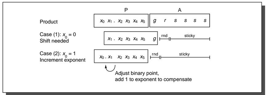
**FIGURE A.10** The two cases of the floating-point multiply algorithm. The top line shows the contents of the P and A registers after multiplying the significands, with  $p = 6$ . In case (1), the leading bit is 0, and so the P register must be shifted. In case (2), the leading bit is 1, no shift is required, but both the exponent and the round and sticky bits must be adjusted. The sticky bit is the logical OR of the bits marked  $s$ .
