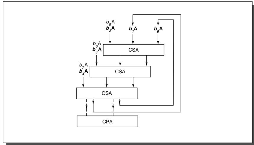
**FIGURE A.28 Multipass array multiplier.** Multiplies two 8-bit numbers with about half the hardware that would be used in a one-pass design like that of Figure A.27. At the end of the second pass, the bits flow into the CPA. The inputs used in the first pass are marked in bold.
