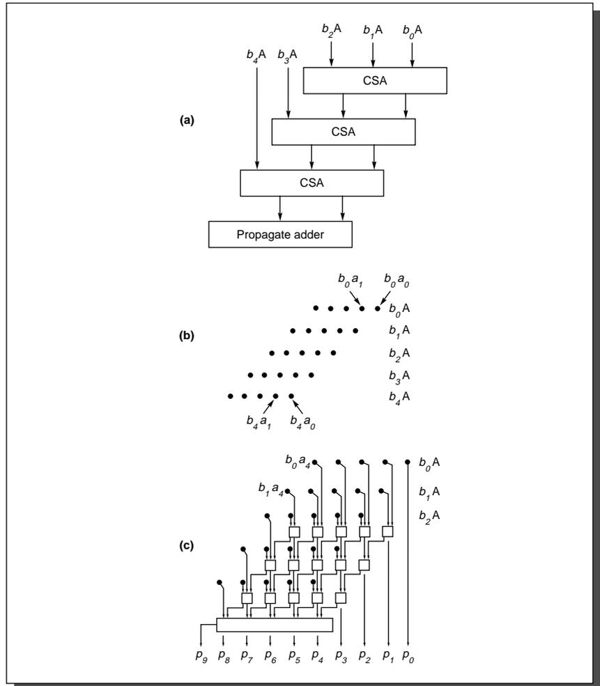
**FIGURE A.27** An array multiplier. The 5-bit number in  $A$  is multiplied by  $b_4 b_3 b_2 b_1 b_0$ . Part (a) shows the block diagram, (b) shows the inputs to the array, and (c) expands the array to show all the adders.
