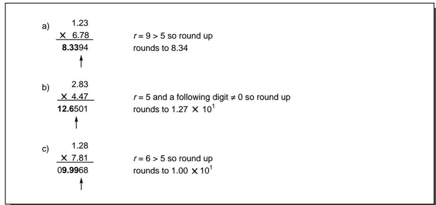
**FIGURE A.9** Examples of rounding a multiplication. Using base 10 and  $p = 3$ , parts (a) and (b) illustrate that the result of a multiplication can have either  $2p - 1$  or  $2p$  digits, and hence the position where a 1 is added when rounding up (just left of the arrow) can vary. Part (c) shows that rounding up can cause a carry-out.
