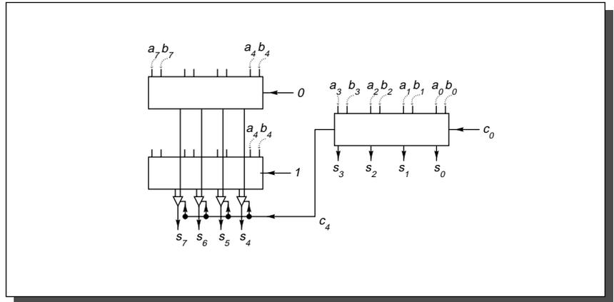
**FIGURE A.20** Simple carry-select adder. At the same time that the sum of the low-order 4 bits are being computed, the high-order bits are being computed twice in parallel: once assuming that  $c_4 = 0$  and once assuming  $c_4 = 1$ .
