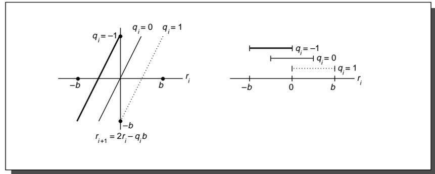
**FIGURE A.32 Quotient selection for radix-2 division.** The  $x$  axis represents the  $i$ th remainder, which is the quantity in the (P,A) register pair. The  $y$  axis shows the value of the remainder after one additional divide step. Each bar on the right-hand graph gives the range of  $r_i$  values for which it is permissible to select the associated value of  $q_i$ .
