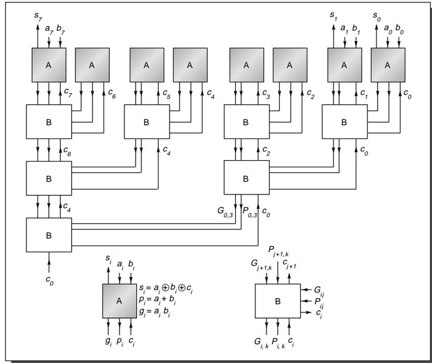
**FIGURE A.17** Complete carry-lookahead tree adder. This is the combination of Figures A.15 and A.16. The numbers to be added enter at the top, flow to the bottom to combine with  $c_0$ , and then flow back up to compute the sum bits.
