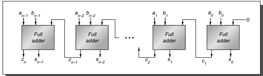
**FIGURE A.1** Ripple-carry adder, consisting of  $n$  full adders. The carry-out of one full adder is connected to the carry-in of the adder for the next most-significant bit. The carries ripple from the least-significant bit (on the right) to the most-significant bit (on the left).
