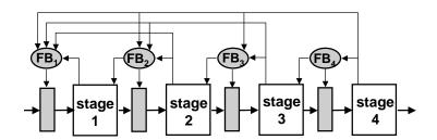
Controlling pipeline in this manner works provided the instruction at stage i+1 can complete without any interference from instructions in stages 1 to i (otherwise deadlocks may occur)
