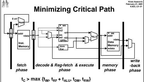
Write-back stage takes much less time than other stages. Suppose we combined it with the memory phase
