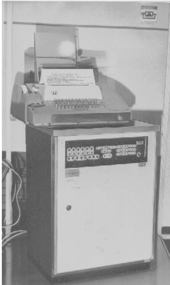
Fig. 5. Microcalculatorul MC-8 (model de laborator) intr-o aplicatie de proces.
