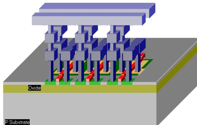
Fig. 15-xxx : 3D View of SOI ring inverter showing the SiO<sub>2</sub> buried layer(inv3Soi.MSK)
