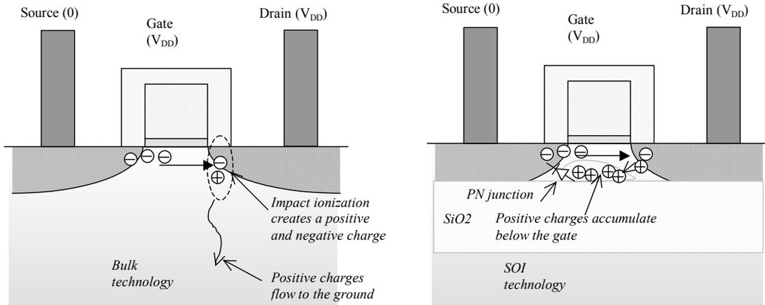
Figure 15-xxx: The impact ionization creates an accumulation of positive charges below the gate in the case of SOI
