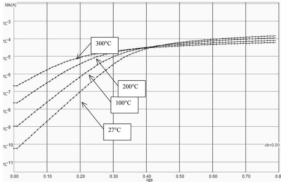
Figure 15-xxx: Temperature effects in SOI MOS devices (Low leakage  $W=10\mu\text{m}$ ,  $L=0.12\mu\text{m}$ )
