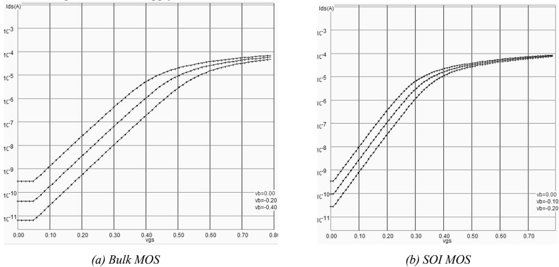
Figure 15-xxx: The steeper sub-threshold slope enables low voltage and low power operations.
