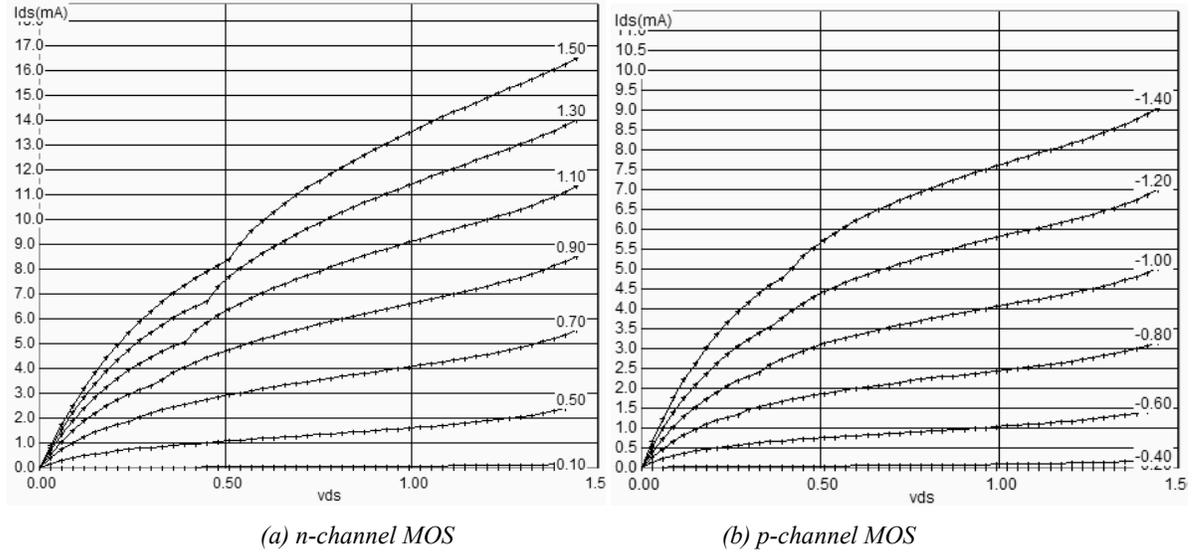
Figure 15-xxx: The drain current characteristics of the n-channel and p-channel SOI devices show a kink effect near saturation
