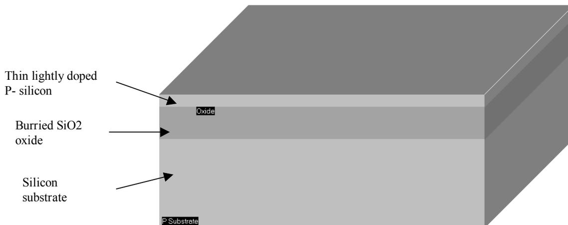
Fig. 15-xxx : 3D View of SOI ring inverter showing the SiO<sub>2</sub> buried layer(inv3Soi.MSK)
