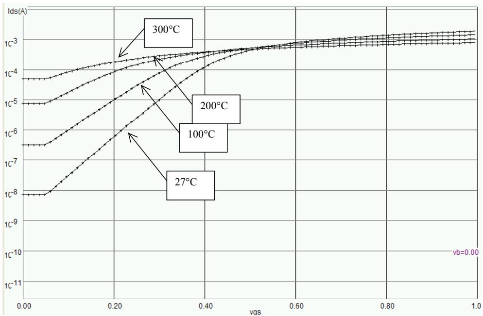
Figure 15-xxx: Temperature effects in bulk MOS devices (Low leakage  $W=10\mu\text{m}$ ,  $L=0.12\mu\text{m}$ )
