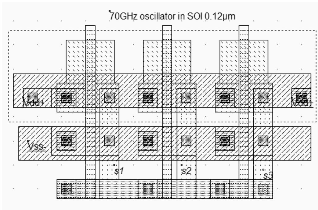
Figure 15-xxx: The ring oscillator in SOI technology (Inv3SOI.MSK)
