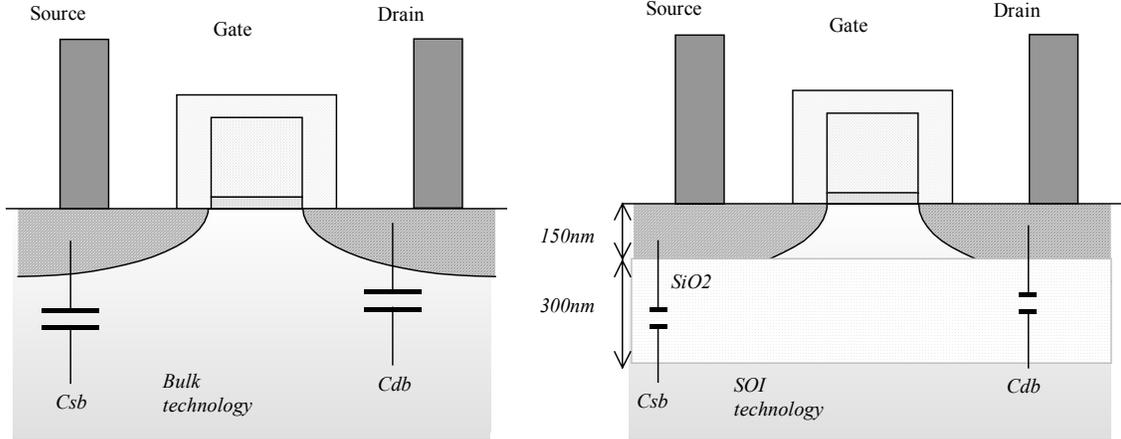
Figure 15-xxx: The junction capacitance between the source and bulk is almost eliminated in the case of SOI.
