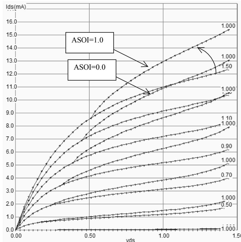
Figure 15-xxx: The effect of the  $A_{SOI}$  parameter on the  $I_d/V_d$  characteristics (Using *soi012.RUL*)
