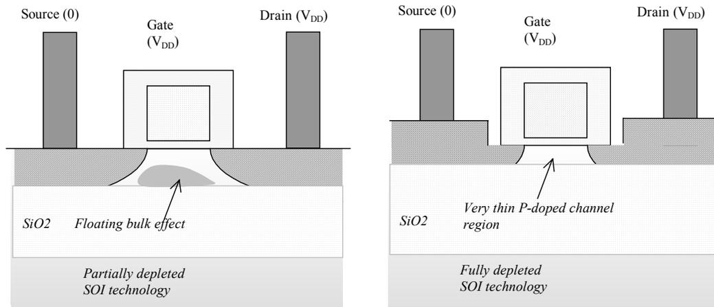
Figure 15-xxx: The fully depleted MOS device has no more Kink effect, but several manufacturing and design drawbacks
