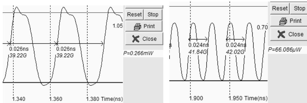
(a) Bulk oscillator at 40GHz: 266 $\mu$ W(b) SOI oscillator at 40GHz: 66 $\mu$ W
