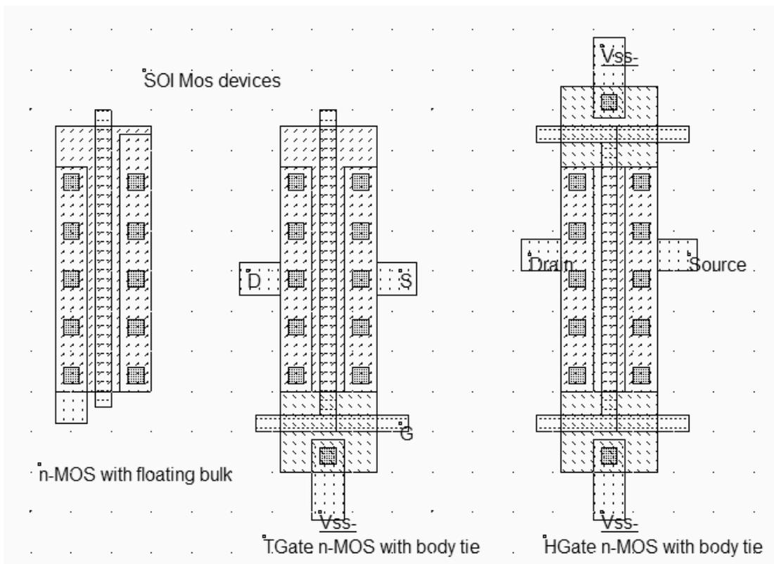
Figure 15-xxx: Adding a contact in partially depleted MOS to avoid the kink effect (mosSoi.MSK)
