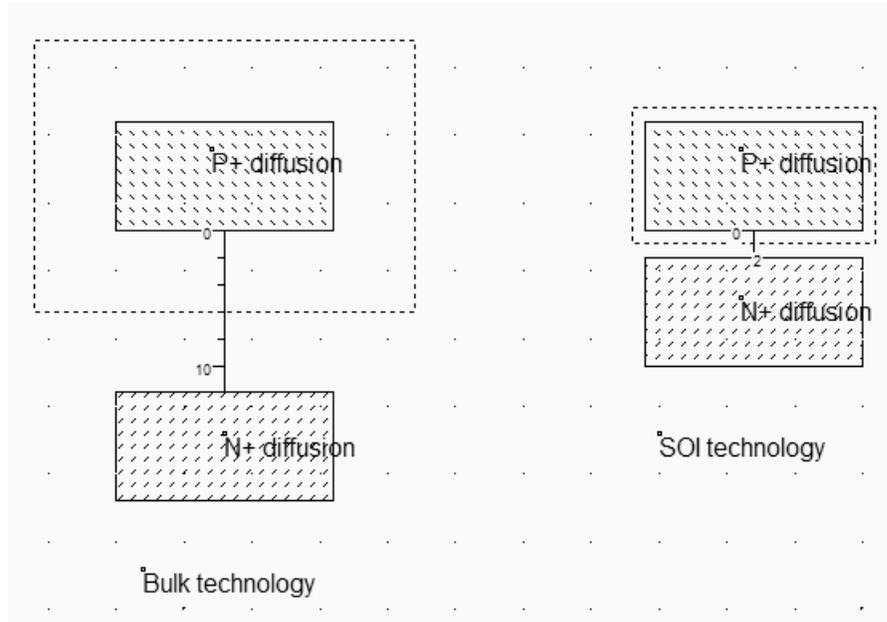
Figure 15-xxx: The increased density due to relaxed design rules between N+ and P+ diffusions (SOIDiffusion.MSK)
